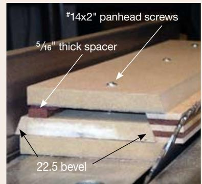
Build this ripping jig from 3/4" MDF, plywood, or particle board. First, rip both edges of the middle layer at the same 22.5-degree angle as the staves. Then glue the middle layer to the lower layer so that one beveled side rides along the saw fence and the other side acts as a support for the previously cut beveled edges of the laminations. Three #14x2" panhead screws provide the clamping pressure and 5/16"-wide strip of hardwood provides a means of leverage. —Malcolm
