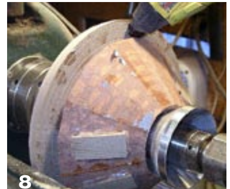
8 A tailstock cone is an ideal centering device.
