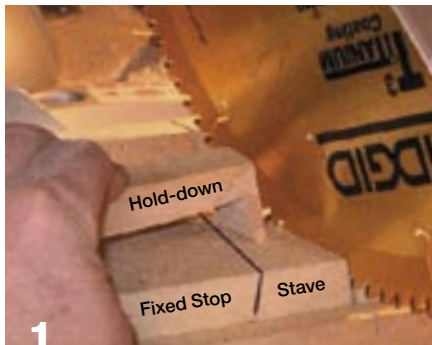
1 Make test cuts to confirm angles.
