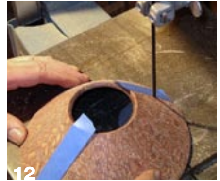
12 Splitting the bowls requires a steady hand. Because the glue line can be difficult to see the blue tape provides a visual aid.
