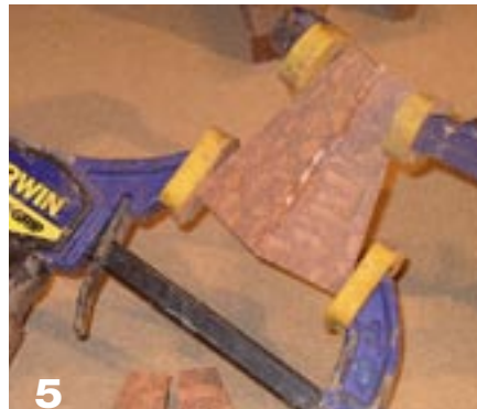
5 Begin gluing pairs of staves.
