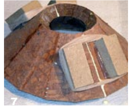
7 Assemble the bowl with the aid of glue blocks and rubber bands.
