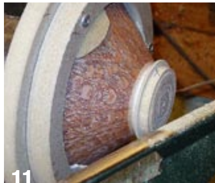
11 Reverse-mount and clean up the small end.
