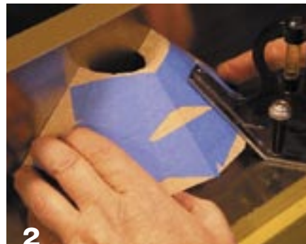
2 At a jointer, check 90- and 45-degree angles.
