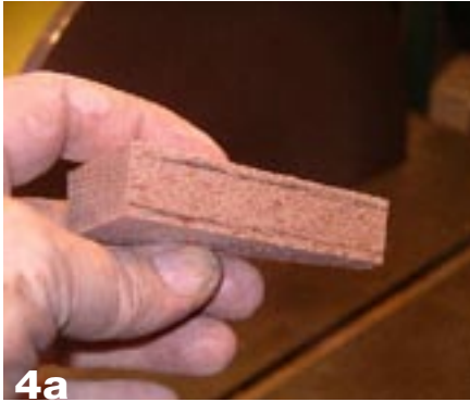
4a To help guide your light sanding, pencil two lines on the edge grain of your staves.
