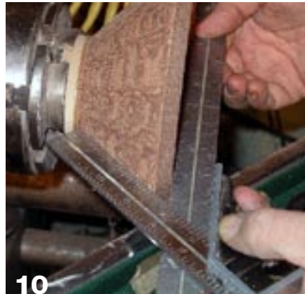
10 Check that the bowl angle is 45 degrees.
