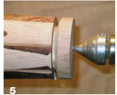
5 After applying glue to the bottom plug, bring up the tailstock to apply clamping pressure.
