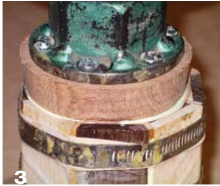
3 Hose clamps provide the ideal pressure for gluing up the stave mug wrap.
