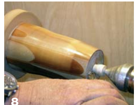
8 With the mug held between a jam chuck and a live center, turn the bottom.
