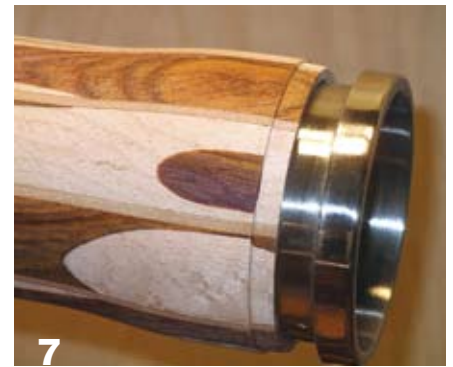
7 Check the fit frequently to get a snug fit between your wrap and the mug insert.
